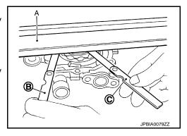
• Calculate the clearance between oil pump inner rotor and oil pump body as follows:
