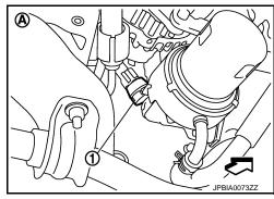
Install the oil pressure gauge [SST: ST25051001 (J-25695-1)]
