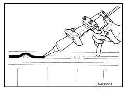
• As for bolt holes (B), normally apply liquid gasket inside the holes. Occasionally, it should be applied outside the holes. Check to read the text of this manual.
